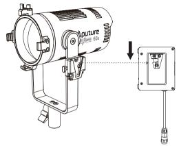
\* To remove the battery case, press the V-mount seat button and pull the battery case upward.
