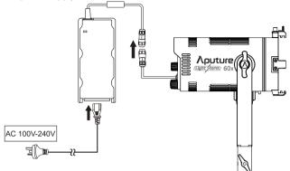
\* Rotate the red rotary ring of the DC input connector clockwise, then pull out to remove the adapter.
