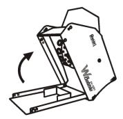
Once the screws are removed, the lid of the housing can be carefully swung upwards, as shown above. Take care not to spill any of the bubble fluid inside the unit.
