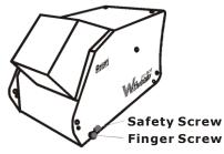
To help avoid accidental exposure to dangerous live AC mains voltage, two safety screws are fitted that require a screw driver to remove. Once these are removed, the finger screws can be undone by hand (see photo above).
