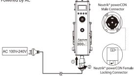
To disconnect the Neutrik® powerCon cable, pull back on the yellow release tab on the cable connector, and rotate the connector counterclockwise.
