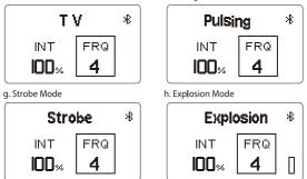
\* In explosion mode, short press the Trigger button to single trigger the light effect.
