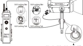
\* Hang the cable from the head cable relief hook to manage and reduce tension on the cable.
