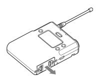
3 Insert two new AA batteries into the battery compartment with ⊕ and ⊖ polarities in the correct orientation, and close the compartment.
