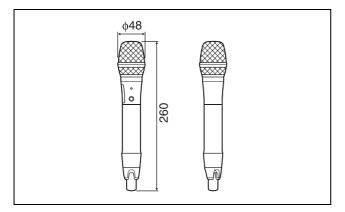
$\phi$  48 × 260 mm (1 <sup>15</sup>/<sub>16</sub> × 10 <sup>1</sup>/<sub>4</sub> in.) (Diameter / length) Approx. 260 g (9.2 oz) (excluding batteries)
