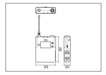
$63 \times 82 \times 20 \text{ mm} (2^{1}/_{2} \times 3^{1}/_{4} \times {}^{13}/_{16} \text{ in.})$
