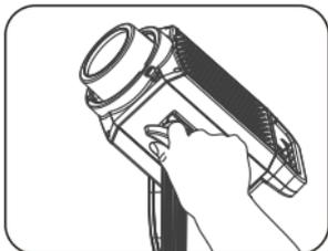
Loosen the angle fixing knob.
