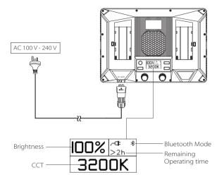
When disassembling the power cable, please rotate the spring lock button on the power cable before disassembling, do not pull it hard.
